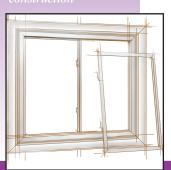
303VS/303BMJ Single Lift Slider NAFS, R-PG50, Water 360 pa, Air - A3, F10 NFRC Certified **AAMA Certified CSA Certified**
